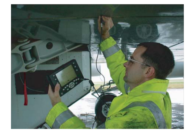
Locator being used to check for corrosion in an aircraft
