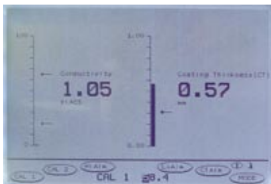
Conductivity & Coating Thickness Measurement Screen
