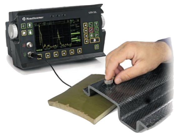
Square wave pulser with tunable pulse width solves composite testing applications.
